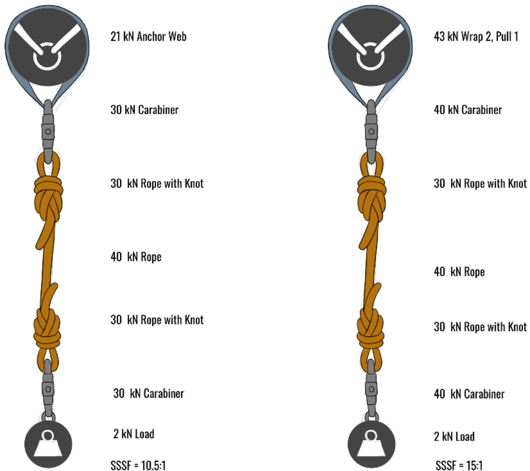
Example 1 of a Simple System 1:1
